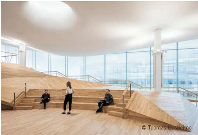
**The ground floor has very little vertical structure, and is column free both inside and out**
