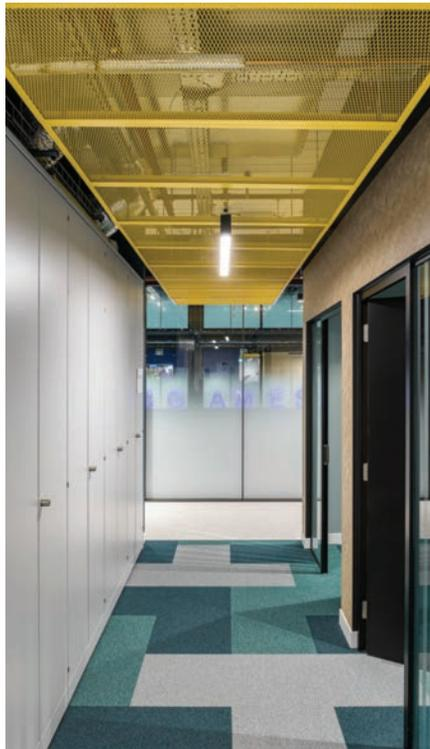
cheap, and relatively acoustically good solution. However, with the option to now use metal mesh in ceilings, a suspended ceiling with benefits including improved airflow, lighting, and vastly improved aesthetics can be achieved.
